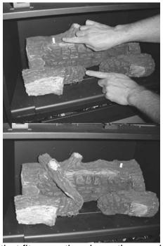
The left twig has a single hole on the bottom that fits over the pin on the rear log. Place the twig as shown above, noting how the twig points towards the center.
