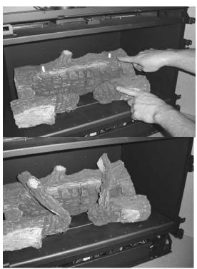
The right twig has a single hole on the bottom that fits over the pin on the rear log. Place the twig as shown above, noting how the twig points towards the center.
