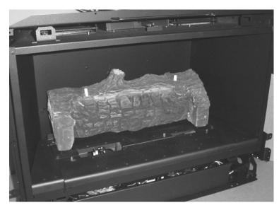
The rear log has two cut-outs on the back edges along the bottom. Place the log on the burner so these cut-outs fit over the two pins on the burner as shown above.
