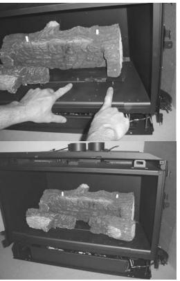
The right log has two holes in the bottom that fit over the two pins on the burner. Place the log as shown above.
