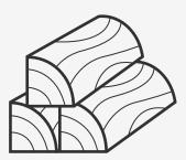
For maximum efficiency and enjoyment avoid burning large pieces of wood and use double split logs (around 10cm diameter max). This will produce nicer flames, cleaner combustion and better heat efficiency.
