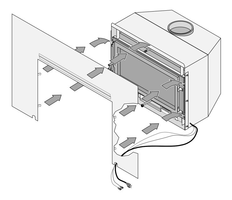
**HINT**: When installing the panel, route the wires through the notch on the bottom of the panel (either side).
