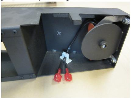
Affix the GreenStart sticker over the hole, and then insert the color-coded start button wires through the hole that the start button should be flush with the trim panel.
