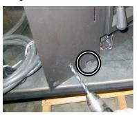
Route the igniter cord through the "mouse hole" in the left side of the panel as shown above. Attach the fathe panel.
