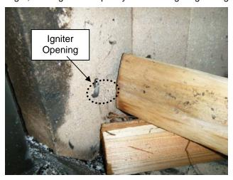
3. Place additional pieces of wood directly in front and in back of the piece of wood placed in step 2. Make sure the wood runs parallel to the igniter air flow and is spaced far enough apart to allow air to flow.
