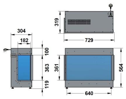
FRAME BUILD OUT DIMENSIONS (All dimensions are in millimetres)
