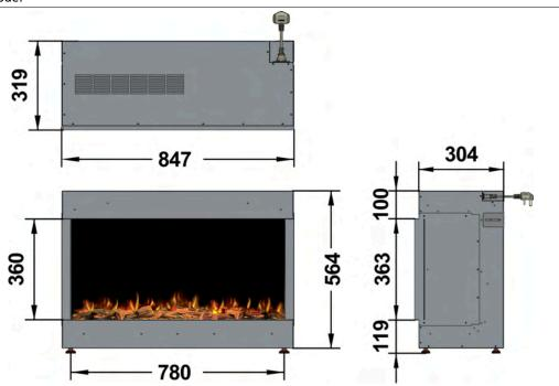
FRAME BUILD OUT DIMENSIONS (All dimensions are in millimetres)
