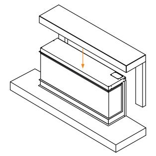
17) Carefully, lower the top section of the surround onto the top of the firebox.
