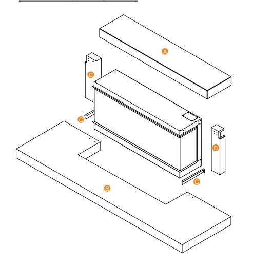
Before Installing the appliance onto the wall with the surround, secure the side trims each side of the appliance as shown below.
