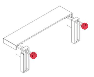
**16)** Screw the two legs of the surround from the rear onto the back of the top section of the surround as shown above
