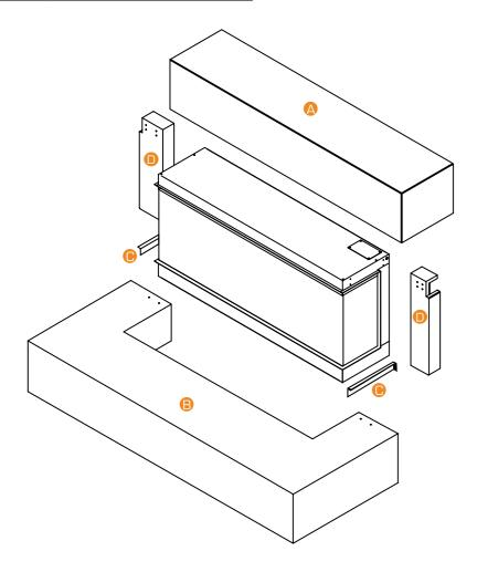
Before Installing the appliance onto the wall with the surround, secure the side trims each side of the appliance as shown below.
