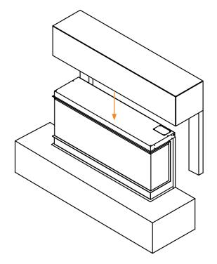
17) Carefully, lower the top section of the surround onto the top of the firebox.
