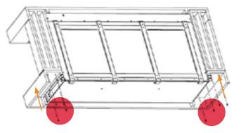
**18)** Underneath the appliance, screw the surround screws up through the bottom surround and into the legs of the surround top section and the other 2 screws either side, up through the bottom of the surround through the floating shelf brackets.
