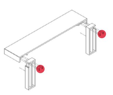
**16)** Screw the two legs of the surround from the rear onto the back of the top section of the surround as shown above
